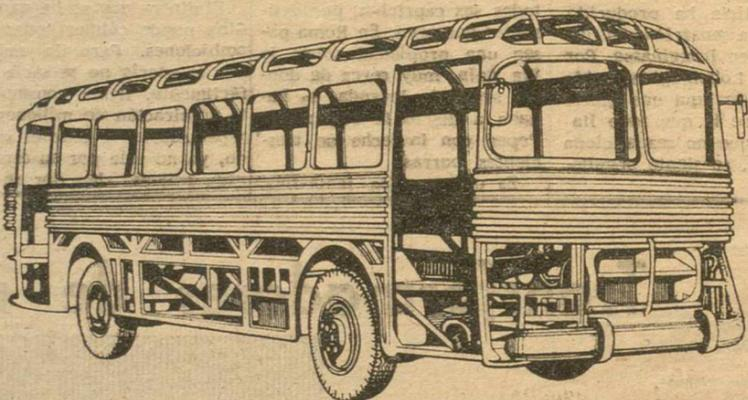
AUTOBASTIDOR: ESTRUCTURA MONOCASCO
