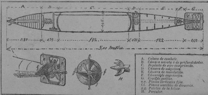
CORTE VERTICAL-LONGITUDINAL DE UN TORPEDO AUTOMÓVIL, SISTEMA WHITEHEAD SCHWARTZ KOPFF, ADOPTADO PARA NUESTRA ARMADA
